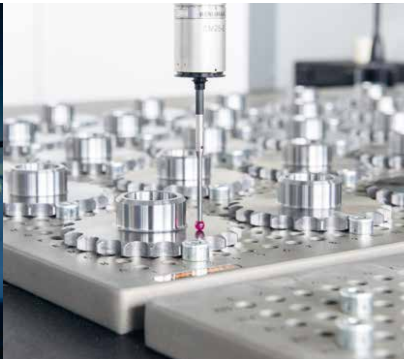
3D sprocket measuring
